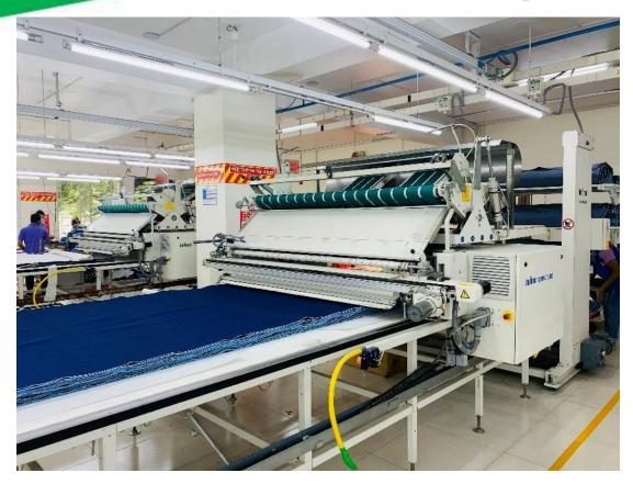
Auto Spreader and Fabric loading facility. It can be use for any kind of Fabric layer
